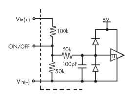
Figure B: Internal ON/OFF pin circuitry
