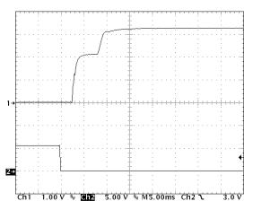
Figure 9: Turn-on transient at full load (resistive load) (5 ms/div). Input voltage pre-applied. Ch 1: Vout (1V/div). Ch 2: ON/OFF input (5V/div)
