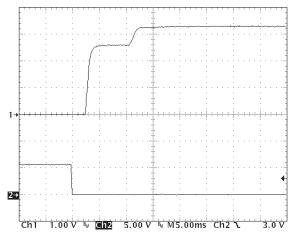
Figure 10: Turn-on transient at zero load (5 ms/div). Ch 1: Vout (1V/div) Ch 2: ON/OFF input (5V/div)
