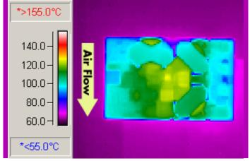
Figure 6: Thermal plot of converter at 23.5 amp load current with  $55^{\circ}C$ air flowing at the rate of 200 LFM. Air is flowing across the converter from pin 1 to pin 3 (nominal input voltage).
