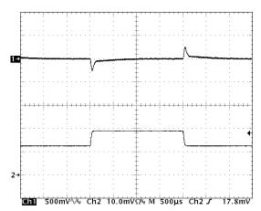
Figure 11:Output voltage response to step-change in load current (50%-75%-50% of lout(max);  $dI/dt=0.16A/\mu s$ ). Load cap:  $10\mu F$ ,  $100~m\Omega$  ESR tantalum capacitor and  $1\mu F$  ceramic capacitor. Ch 1: Vout (500mV/div), Ch 2: lout (10A/div).
