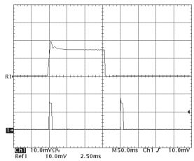
Figure 18: Load current (20A/div) as a function of time when the converter attempts to turn on into a 1 m $\Omega$  short circuit. Top trace (2.5ms/div) is an expansion of the on-time portion of the bottom trace.
