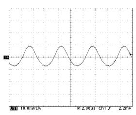
Figure 14: Input Terminal Ripple Current, ic, at full rated output current and nominal input voltage with  $10\mu H$  source impedance and  $47\mu F$  electrolytic capacitor (500 mA/div). See Figure 13
