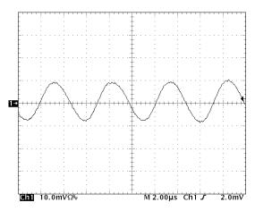
Figure 15: Input reflected ripple current, is, through a 10  $\mu$ H source inductor at nominal input voltage and rated load current (10 mA/div). See Figure 13.
