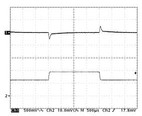
Figure 12: Output voltage response to step-change in load current (50%-75%-50% of lout(max):  $dI/dt = 0.4A/\mu s$ ). Load cap:  $470\mu F$ ,  $30 \text{ m}\Omega$  ESR tantalum capacitor and  $1\mu F$  ceramic cap. Ch 1: Vout (500mV/div), Ch 2: Iout (10A/div).
