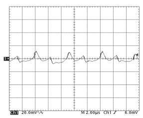
Figure 16: Output voltage ripple at nominal input voltage and rated load current (20 mV/div). Load capacitance: 1µF ceramic capacitor and 10µF tantalum capacitor. Bandwidth: 20 MHz. See Figure 13.
